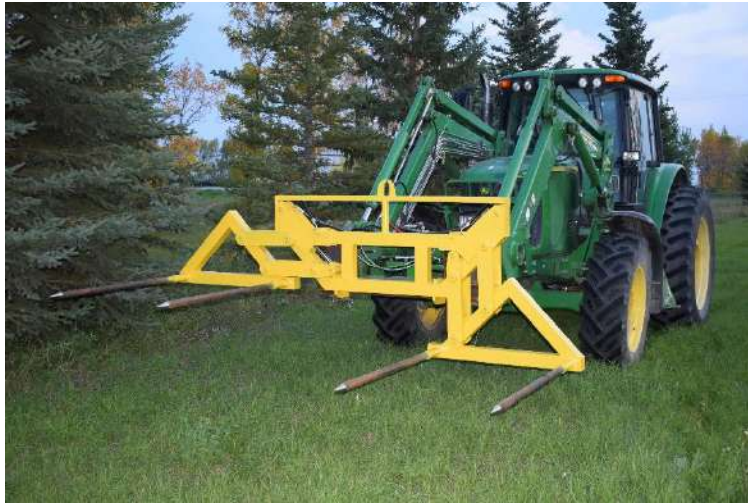
Figure 3 One Fork Lifted ready to spear second
